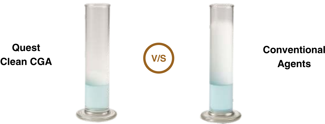
Comparison of foam production for Quest BioClay based chemistry vs competition
